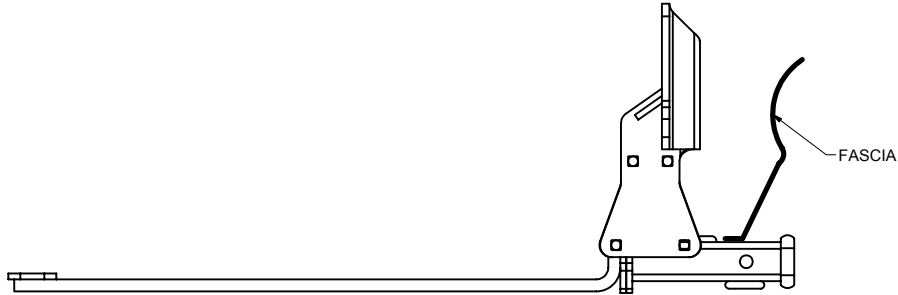
INSTALLED HITCH POSITION
