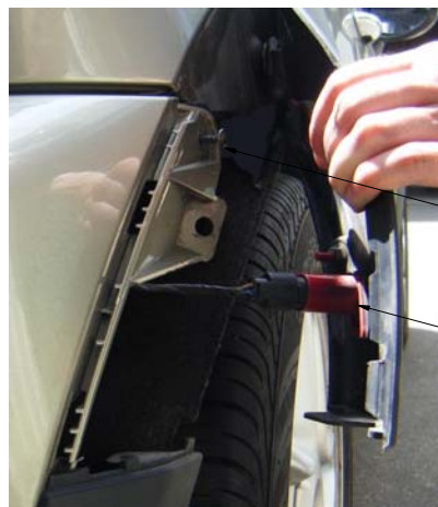
Photo 4: Fastener C behind wheel moulding.
