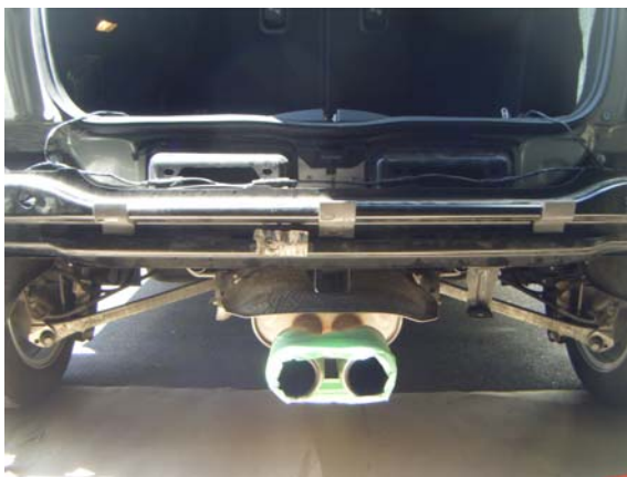
Photo 8: Hitch and Bumper Beam Installed
