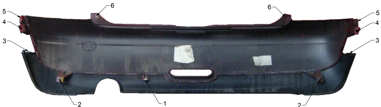
Photo 2: Fastener locations as viewed from inside of the bumper cover. (These fastener locations are present on all models.)
