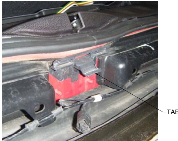
Photo 5: Tab located at center of hatch under the bumper cover.
