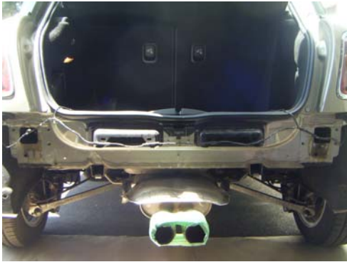
Photo 6: Bumper beam removed.
